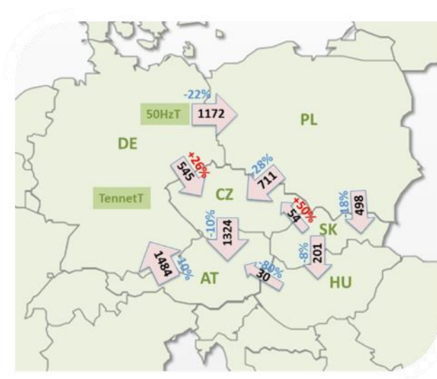
Figure 2. Average annual volume of unplanned power flows on the Polish borders and some other borders in the region of Central-East Europe in 2016 [MW-h] as well as change in this volume in comparison to 2015 [%]
